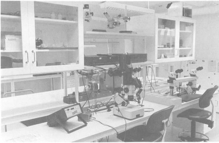
FIG. 5—A stereo microscope with the color camera and a panel with six video connection points.
